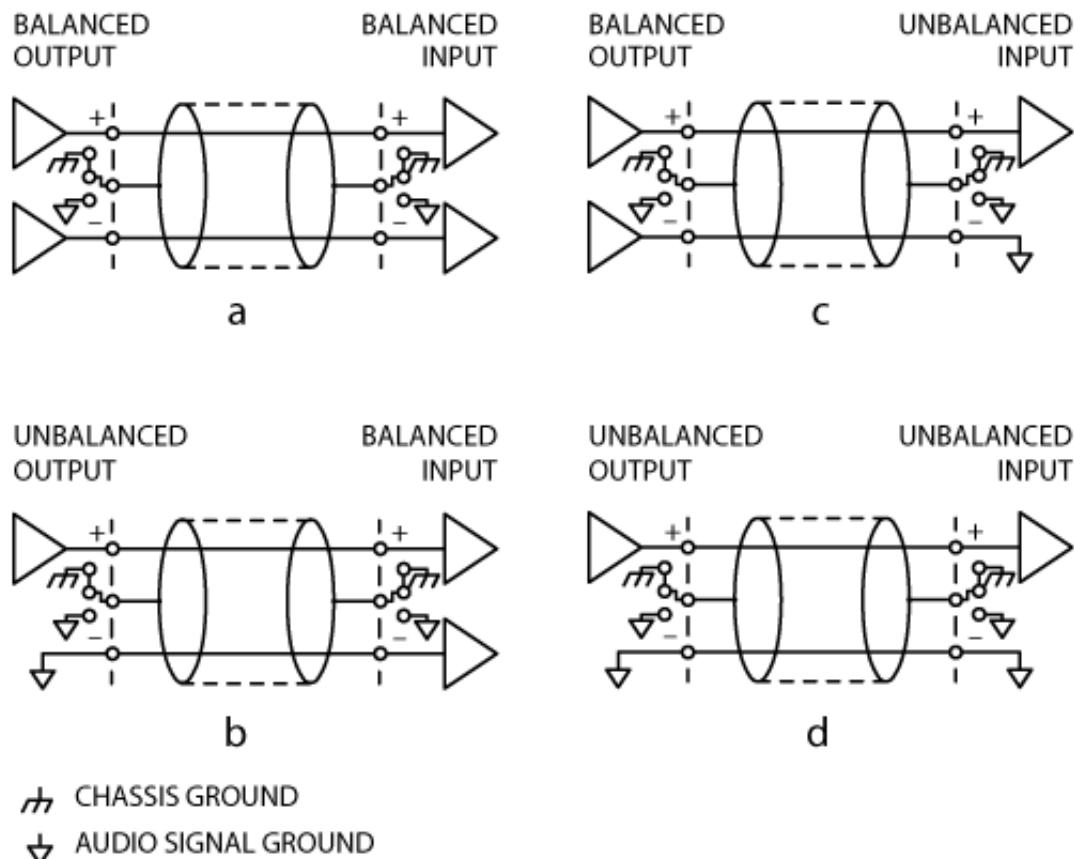
**Figure 8. User-Selectable Shield Connections.**
