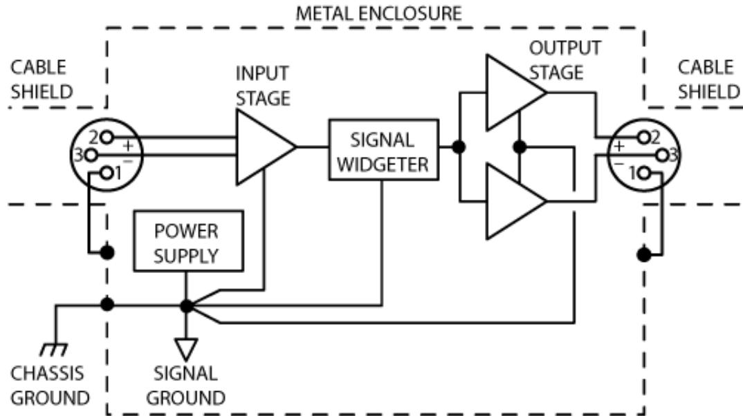
**Figure 4. Star ground scheme for connecting signal ground to chassis. Star center may be connected at power supply, or at input ground.**
